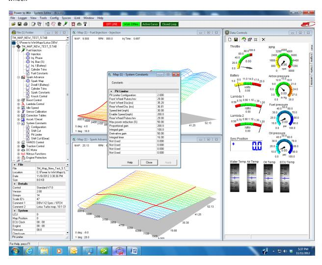
Note: If logging wheel speed and want to see the actual MPH (not what is multiplied to offset the stock dash), a Math Channel must be created. I.e. Name 'Front Wheel MPH', equation = (Frontwheel/1.6). Repeat process for Rearwheel channel. Math Channels are explained in more detail in the Math Channels documentation. Vehicles using aftermarket displays should have wheel diameters entered in actual inches. Then if desired to log channels in MPH select 'Imperial' units and for KPH select 'Metric'.
