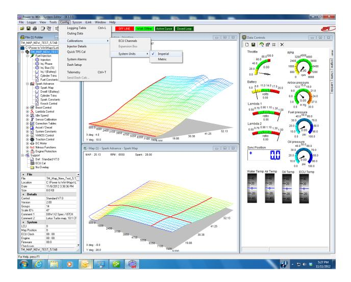
Maps for U.S. vehicles that are supplied by DRS will come with the wheel speed diameters multiplied by 1.6 in order to offset the data the dash receives. ECUs are also pre-configured for this before leaving DRS. In the event that your logger has been reset this procedure may be required. The "Config" file lives in the PC interfacing with the ECU, not the map. If your map needs the speed to be fine tuned for your tire size this can also easily be done.
