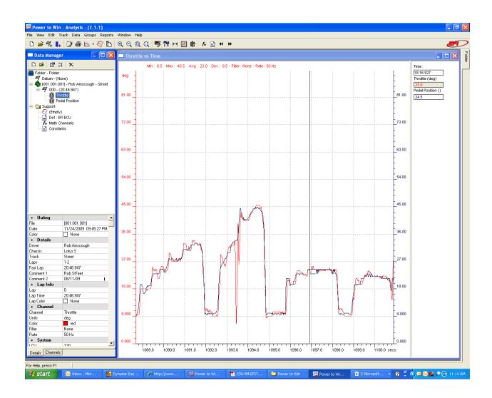
Channel details can be adjusted, such as decimal placement, Upper and Lower Scales, and Filters.
