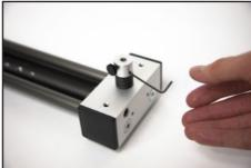
4. Screw in Coupler into the holes of the shaft.
