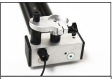
16. Screw in Quick Release Motor Mount.
