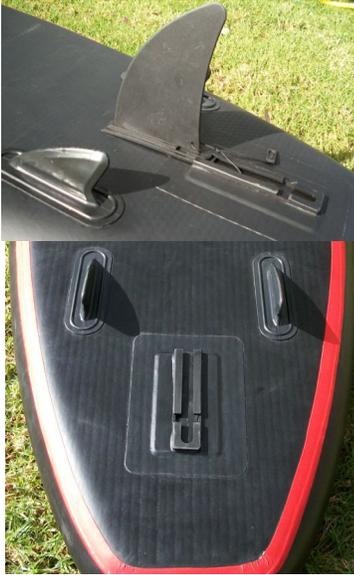
2) Clean & Dry the Board: With the valve unit still closed, rinse off the board with fresh water. Dry around the valve unit with a towel. Allow the red EVA pad to dry thoroughly before rolling for storage.
