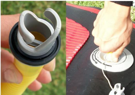
5) Inflate Board: Pump air into the board. Take note that the pressure gauge may not register air until the board reaches 10 PSI. Board will take form in 4 mins/100 full pumps. Once the desired PSI is reached (15 PSI = 225 pumps), remove the hose to replace the valve unit cap.
