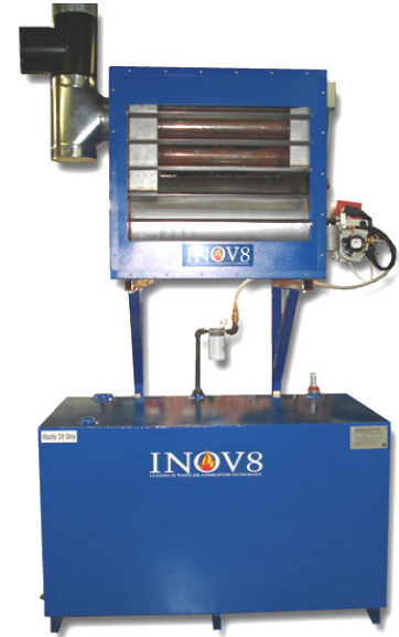
Photo shows a completed installation of a model F240 mounted on an INOV8 model T300 tank with a chimney, oil lines and gauge. Note that the brackets have been shortened.
