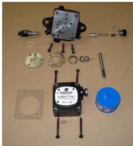
Pump – showing all internal parts
