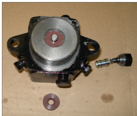
Pump showing seal
