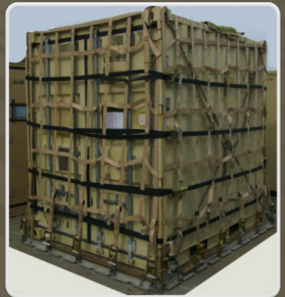
Corner View: Short & Long Sides with ratchets for vertical adjustments. On the corner are the horizontal adjustable straps with ratchets.
