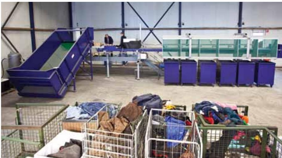
Engineers operate the newest textile sorting NIR spectrometer in the center of the image. Courtesy: Wieland Textiles B.V., Wormerveer, The Netherlands
