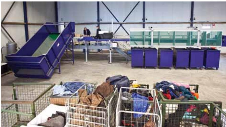
Engineers operate the newest textile sorting NIR spectrometer in the center of the image. Courtesy: Wieland Textiles B.V., Wormerveer, The Netherlands
