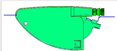
Place the cam in the approximate position as shown and thread the mainline through LongLiner as it appears here. The cam side of LongLiner points toward your bait or lure and the narrow side toward your rod. LongLiner will now free slide on your main line.
