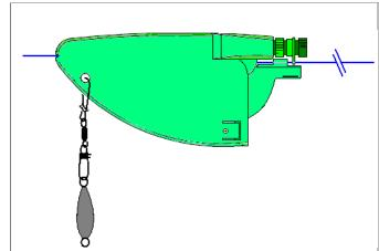
While the boat is underway, hold LongLiner in hand and let your bait or lure trail behind the boat taking line off of your spool. Manually pull line through LongLiner if the lure is small. When the bait is at a distance from LongLiner or boat that meets your satisfaction, lock the cam into place and let LongLiner into the water and down to the desired depth. See our package or online chart for depth control.
