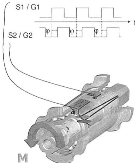
**Figure 1** — The optoelectronic sensor of the Ergomo®Pro power meter.
