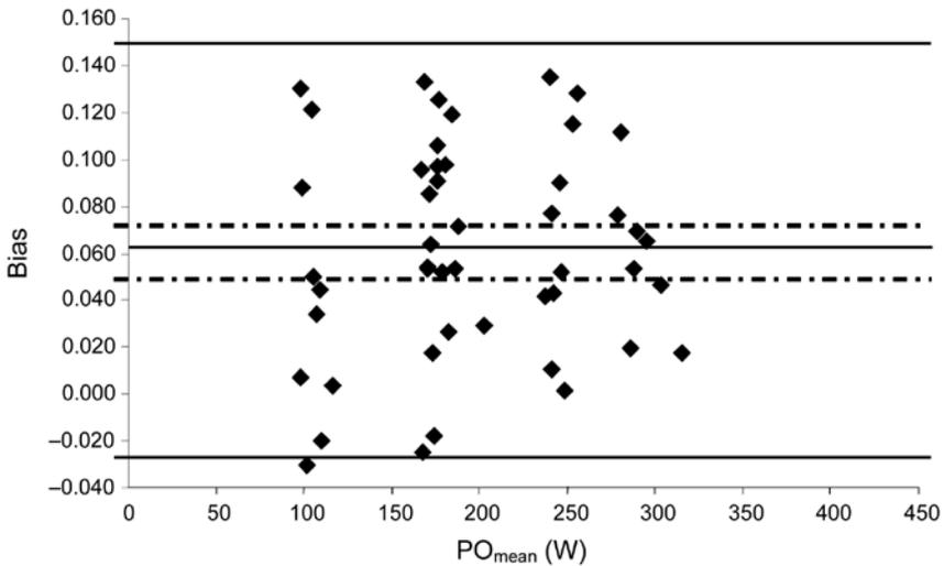
**Figure 3**— Bias (center line), limits of agreement (continuous line), and 95% confidence interval (dashed line) obtained with Bland–Altman analysis for the comparison between the power outputs (PO) measured on the Ergomo®Pro (EP) and SRM power meters during the 8 submaximal incremental tests.  $PO_{\text{mean}} = (PO_{\text{EP}} + PO_{\text{SRM}})/2$ .
