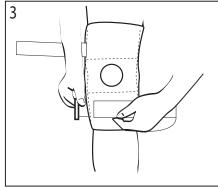
Secure Lower Strap Wrap lower strap around the brace, then loop strap through D-ring. Pull strap back to tighten and press tab end to secure
