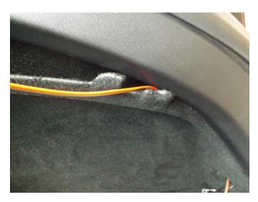
**Step 11.** Once the wire has been threaded through the hole on the underside of the side panel, align the ELLuminer LED strip on the bottom side of the plastic Tesla Parcel Shelf bracket running along the side, it is a personal preference in positioning the LED strip.
