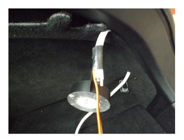
**Step 9.** Remove the tape attaching the ELLuminer wire from the Romex cable. The connector end is ready to be reconnected to the New ELLuminer LED light assembly, plug it in to the new LED, push the wires into the hole, and replace the LED assembly in its hole.
