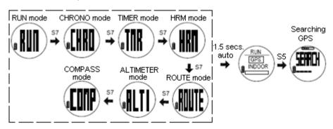
**4.3.3)** Press and hold S7 for 2 seconds from any mode while GPS is initially **OFF**.
