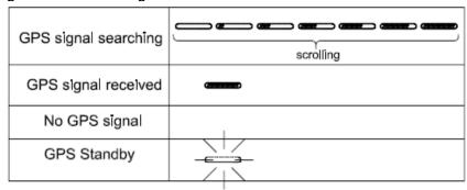
You will hear a beep sound when the Watch has received a GPS signal or when the GPS signal has been lost. LOST GPS signal will also be displayed in the screen.
