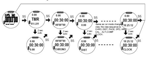
**6.3.4.** Ho to view the TIMER segments while the chrono is in reset view: Press S5 while in GPS GO screen then press S11 to toggle timer segment 1 to 6.
