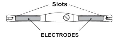
**5.3.** Wrap around the chest belt around your rib cage just below the pectoral muscles and attach the other end of the strap to the HRM transmitter. The elastic strap should be adjusted so that it is snug enough so that it will not move during use but not so tight as to restrict breathing.
