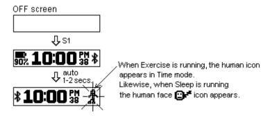
Note that this device has an auto OFF screen function. Press any of the buttons will turn ON the screen.
