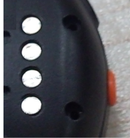
4 contacts at the back of the watch
