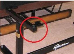
5.) Line up the threaded holes on the Equicizer's frame to the Riser Stand foot plates. Riser Stands bolts are still loose to help line up the Riser Stand to the Equicizer's frame. Line up one plate at a time and place bolt with washer under Riser Stand foot plate and hand turn to get started. DO NOT TIGHTEN until all 4 bolts of Riser Stand foot plates are attached to the Equicizer Frame.
