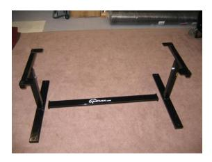
2.) Assemble the cross brace of the Riser Stand using the bolts that are in place. DO NOT FULLY TIGHTEN ANY OF YOUR BOLTS YET!
