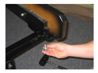
6.) Once all 4 bolts are loosely in place tighten all 4 bolts completely.
