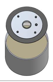
PUSH FOLLOWER PLATE INTO THE BUCKET AND ENSURE IT RESTS FLAT ON THE SURFACE OF THE BULK MATERIAL
