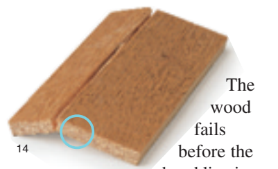
After staining, the bond line is hard to find. Look inside the circle.
