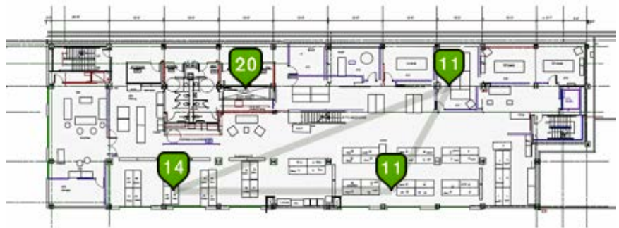
Figure 22 - Good AP Deployment for Accurate Location
