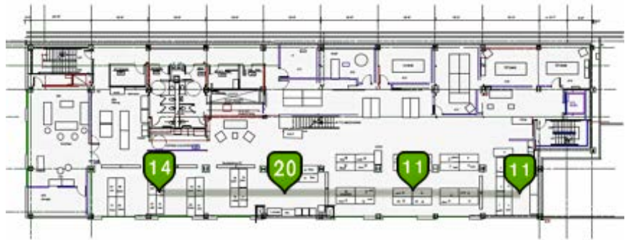
Figure 21 - Poor AP Deployment for Accurate Location
