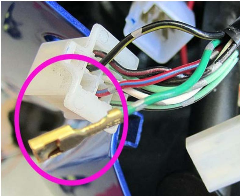
Image of the green wire pulled out. Notice how the tab is bent inwards now that you have removed it.
