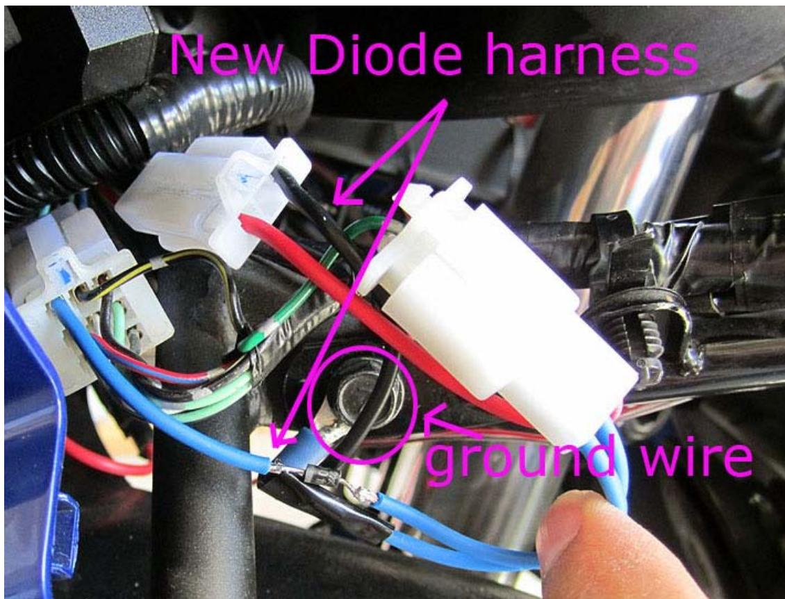
Pic of the new kit installed with the ground wire attached.
