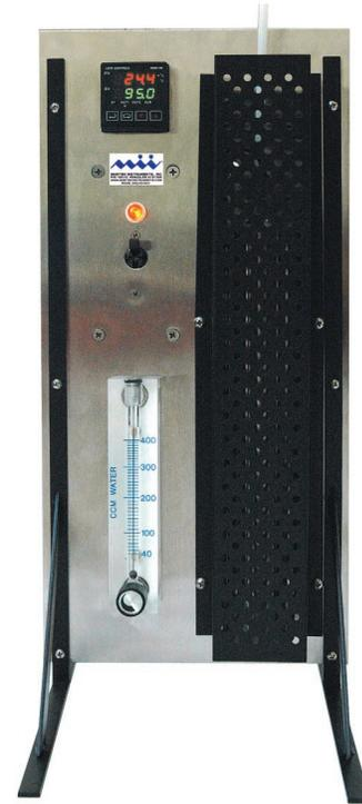
the process solution to near-boiling after a cation column, carbon dioxide and other low molecular organics are volatilized and removed. Differential analysis between cation and degassed conductivity measurements can provide a more accurate cation conductivity value that can be directly correlated to CO<sub>2</sub> concentration and result in a more realistic assessment of the process chemistry.
