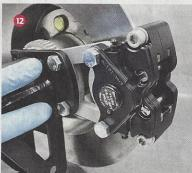
attach the caliper to the bracket then bolt the assembly to the arm.)
