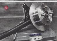
\*Note, the factory rear-trailing arm shown has the e-brake cable cut. The e-brake cable will have to be removed from the handle (inside the car) before the OEM rear trailing arm can be removed.
