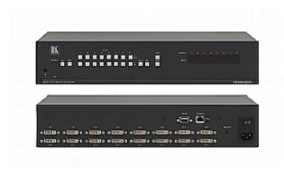
The VS-88HDCPxI is a high-performance matrix switcher for DVI and HDMI signals on a DVI-D connector. It reclocks and equalizes the signal and can route any input to any or all outputs simultaneously.
