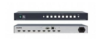
The VS-81H is a high-performance switcher for HDMI signals. It reclocks and equalizes the signal and switches one of the 8 inputs to a single HDMI output.
