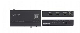
The VS-21H-IR is a high-performance switcher for HDMI signals. It reclocks, equalizes and switches either of two inputs to a single HDMI output.
