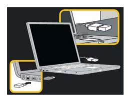
Insert the USB Dongle into the computer - For best results use a USB extension cable.
