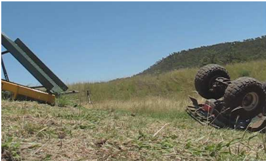
Figure 10. Moto 250 at rest after low speed back flip – without Quad Bar
