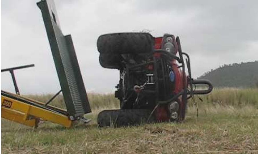
Figure 12. Test 1746 with Cattleman ATV resting on side at the end of the roll sequence
