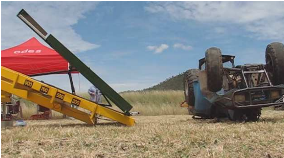
Figure 5. Test 1665 with ATV upside down after half roll
