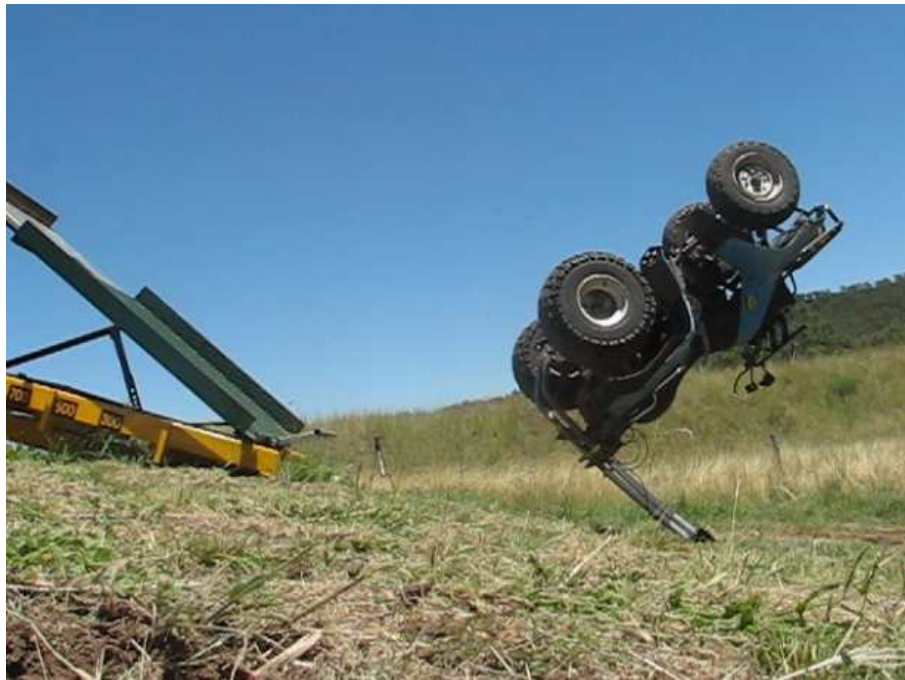
Figure 9. Moto 250 at highest point during potential back flip
