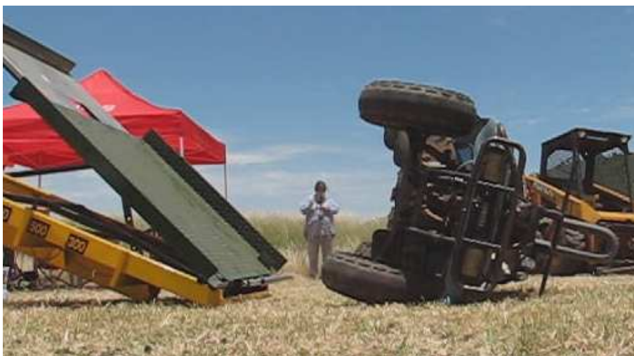
Figure 8. Test 1673 with ATV resting on side at the end of the roll sequence
