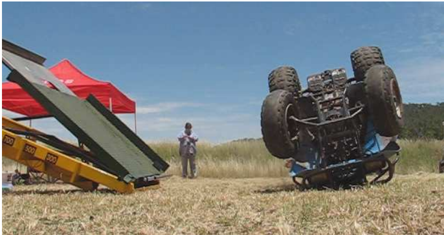
Figure 7. Test 1673 with ATV inverted part way through the roll sequence (with large space between the seat and the ground surface)
