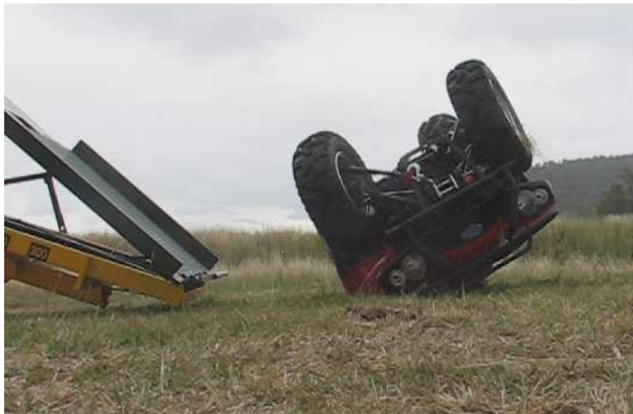
Figure 11. Test 1745 with Cattleman ATV resting upside down at the end of the roll sequence
