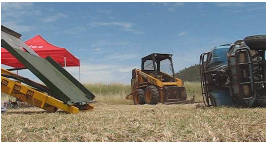
Figure 6. Test 1670 with ATV on opposite side after three quarter roll
