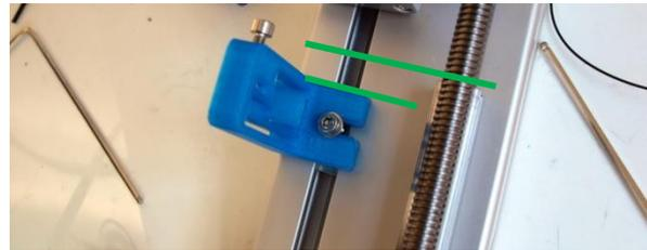
Mount the z-axis-limitswitch vane with an m4x20 bolt + washer. The bracket should be approx. 1cm from the top of the rail. This is the adjusting mechanism for the z-axis height and will be covered later for finetuning.
