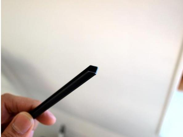
Cut a piece of 20cm from the frame strips. Remove sharp edges, to prevent damage to cables.
