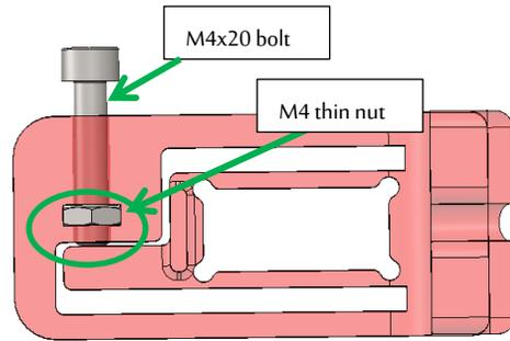
Take the z-axis\_limitswitchvane and slide the nut into the slot. On top screw in an m4x20 bolt. Don't screw it all the way in, let the tip of the bolt touch the flange as indicated in the picture.
