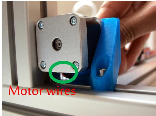
Before mounting the motor make sure the wires are orientated as above
