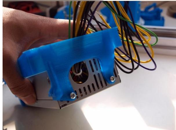
Mount the electronics case base part onto powersupply with the powersupply screws (short thick philips head screws). Slide the part on the powersupply from the top.
