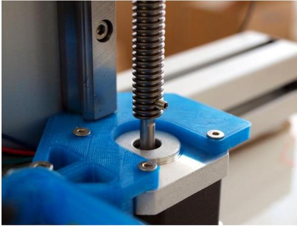
**CAREFULLY** Screw in the z-axis spindle from the top until it reaches the motor and place the z-axis assembly in the middle. Make sure the brass nut is inside the z-axis carrier assembly.
