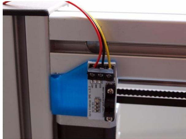
Take the 3 wire cable and mount it onto the sensor as shown above.
