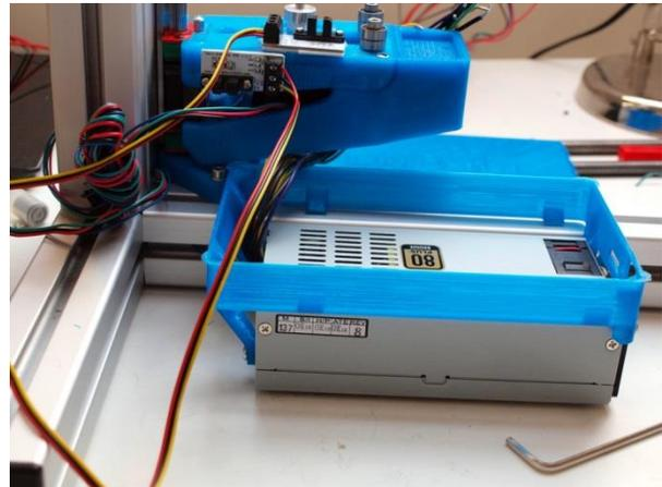
Mount the wires for the opto-sensors of the y and z-axis.
