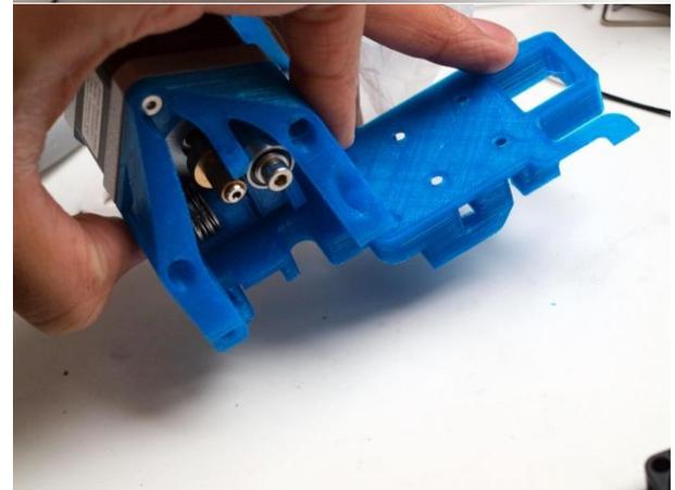
Slide the motor-subassembly onto the base.
