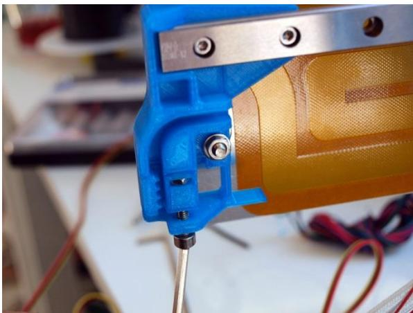
Mount the y-stage bracket pt4 onto the y-stage bracket pt6 with an m4x25 bolt.
