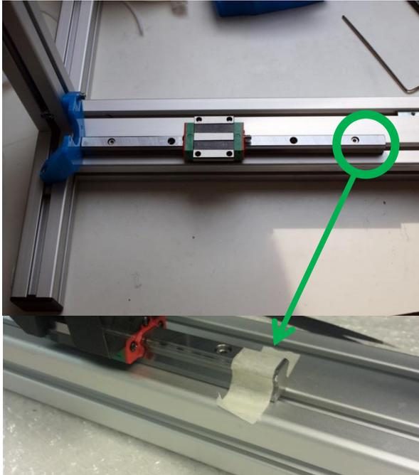
Put some tape on the far edge of the rail to prevent the cart from sliding off.
