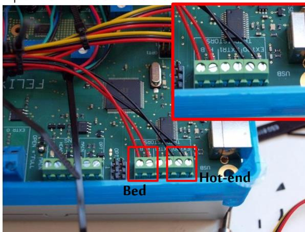
Connect the thermistors (temperature sensor) of the heated bed (red wires) and hot-end (black wires)
