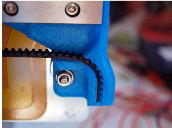
Push the belt inside the bracket. Let the belt make contact with as much teeth of the bracket as possible. Also push it as far as possible, use a small allen key for that. If you have misplaced the belt or you want to remove it, on top of the bracket is a small hole which can be used to push out the belt with a small allen key.
