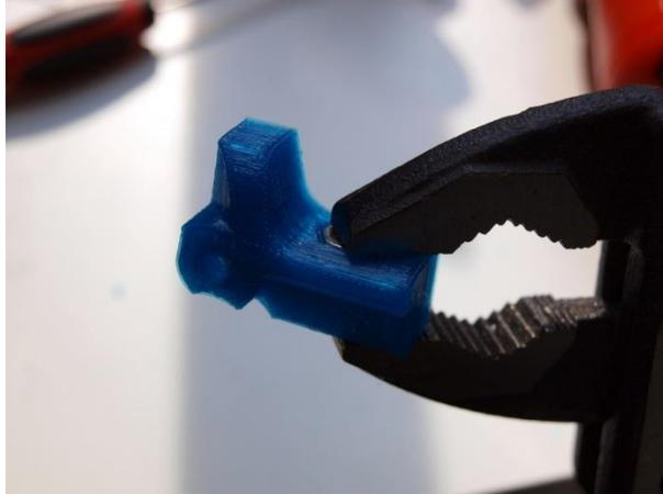
Insert a thin nut m4 as shown above. Before doing that clean the hole out a little and insert the nut.
