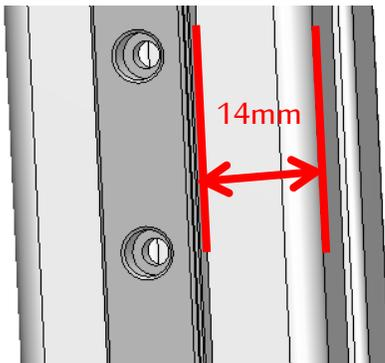
The distance along the rail and the edge of the beam should be 14mm. This way it is centered perfectly over the slot of the beam.
