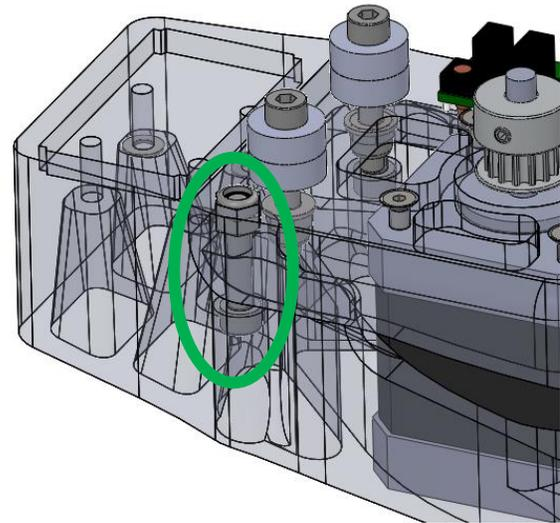
As indicated screw on both sides m4x20 bolts into the part to clamp the 2 big plastic parts together.
