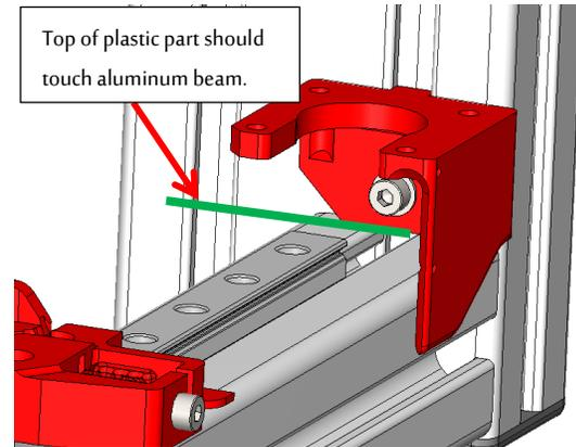
Mount the x-axis motor bracket onto the frame with an M4x16 bolt, use a small washer underneath the bolt-head.
