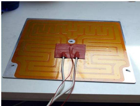
The goal of this module is to get the foil heater onto the aluminum plate. The picture above shows the back/bottom side of the plate.
