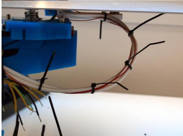
Make a loop as indicated above. Make sure that when moving the table from one side to the loop is just long enough. Make use of cable ties to better form the loop. They can easily be removed later on.
