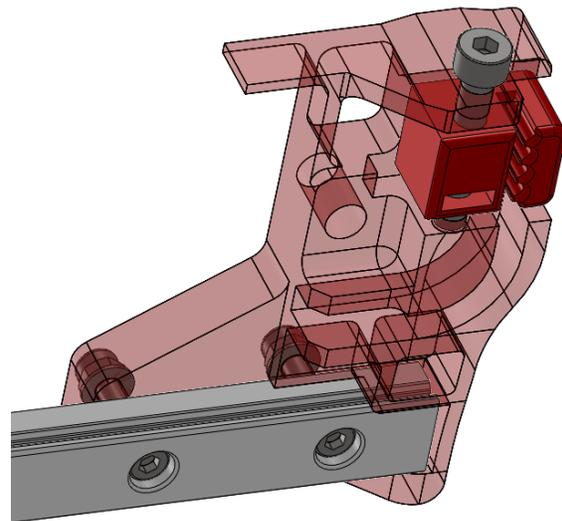
Mount both brackets onto rail with m4x16 bolts and the m3 self locking nuts. Don't forget to place the washers
