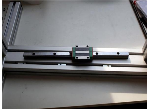
**IMPORTANT: DO NOT** let the cart of the linear bearing go off the rail. There are small balls in there which might fall out when the cart rolls of the rail.
