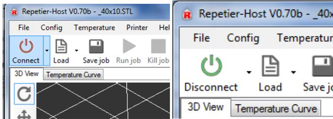
Other checks to see if the printer is connected properly:
