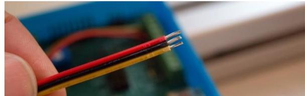
Take the wires of the x-axis opto-sensor, strip the ends.
