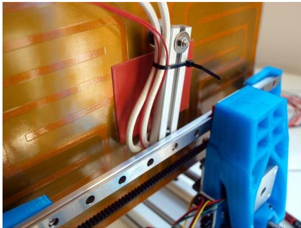
Guide the cables of the z-axis table like indicated above. Make sure the wires are mounted to the small aluminum beam as indicated above. This provides tension relieve to the wires.
