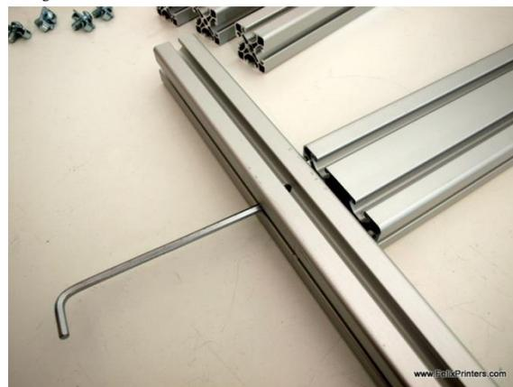
Slide beam 4 in position. On the side of beam 1 where the hex-key is positioned there are two drilled holes. Tighten the frame connectors by
