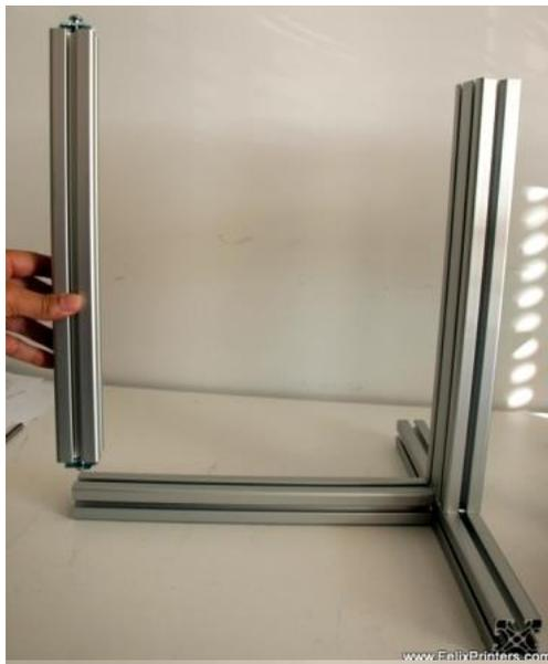
Take beam 2 again and screw the frame connector on it's far end. Then slid it on beam 3 as indicated on the picture.
