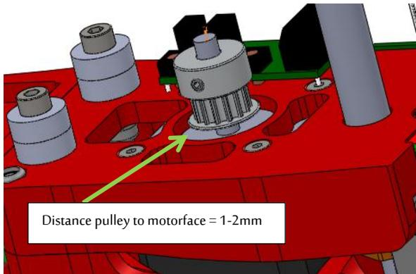
Place the pulley upside down on the motorshaft. The distance of the bottom of the pulley to the faceplate of the motor should be 1-2mm.
