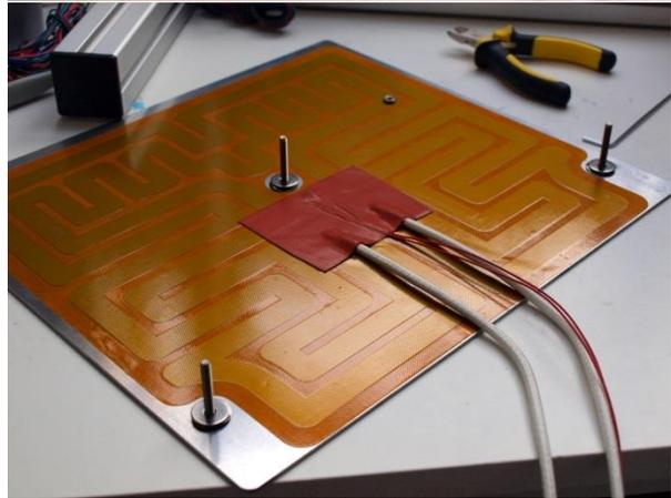
Take the table assembly and place the m4x30 countersunk bolts as indicated above on the three holes in the table. Put a curved washer, large washer and fix those with a m4 thin nut.
