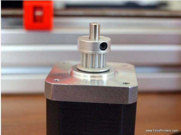
Mount a pulley onto the motor-shaft upside down. The distance between the bottom of the pulley and the face of the motor should be approx 0.5mm, this can be adjusted later on if required.
