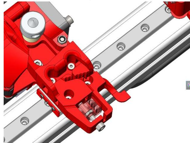
Mount the extruder assembly onto the cart of the linear guide, with 4 m3x6 countersunk bolts.
