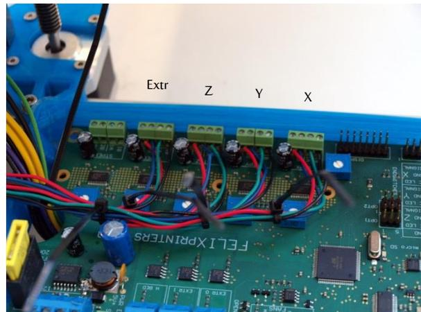
Do this for the rest of the motor wires. Note the cable ties.
