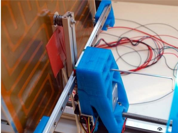
Re-orientate the frame by placing the wide beam onto a table. Mount the y-axis cart on the z-axis part with four M3x16 bolts with the m3 washers.
