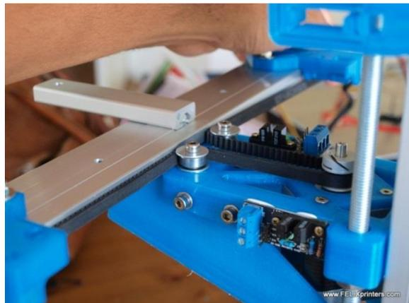
Guide the belt over the pulley and 2 bearings as indicated above.
