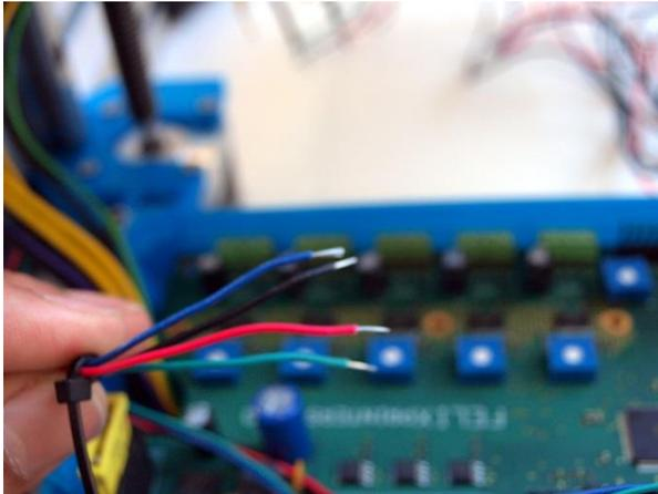
All wires have to be screwed under a screw terminal. These are the steps:
