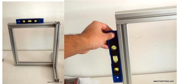
Now it is time for fine-tuning. Try to get every beam as level as possible. Also align the beams as good as possible. See an example in the picture below
