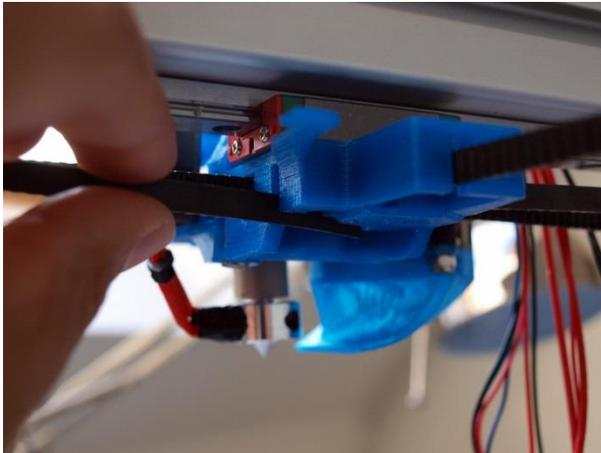
Guide the belt over the motor pulley back to the extruder carriage and insert it in the toothed slot
