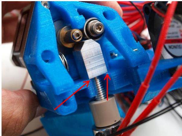
Move hot-end into slot and make sure edge of hot-end touches the base of the extruder.
