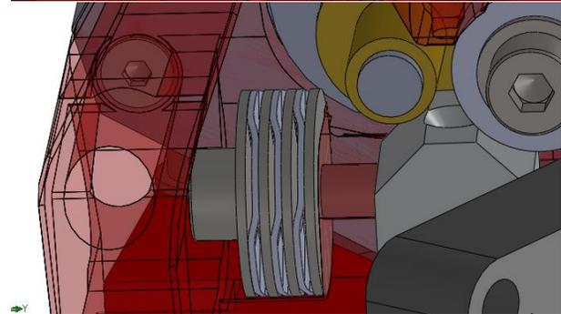
Mount the extruder arm onto the just mounted parts. An m4x40 bolt is required. Use 4 large washers and 3 curved washer as shown in the picture above. **NOTE: Make sure the bolt goes straight into the nut!**
