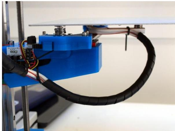
Remove the cable-ties which hold the loops together. Now put the cable spiral around it and cut to length.
