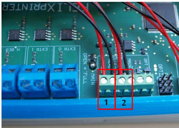
Connect the wires of the fans.
