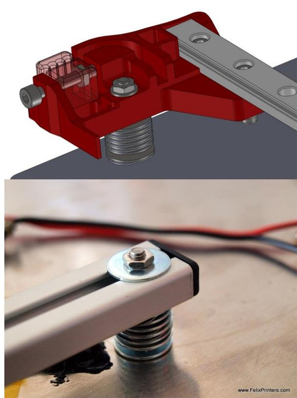
After placement mount table bolts with an M4 thin nut. Use a small washer underneath the m4 nuts at the plastic parts. Use a large washer for the bolt at the small aluminum beam.
