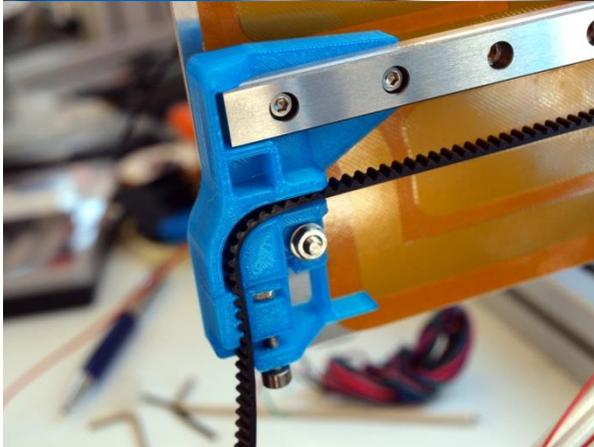
Push the belt into the small printed clamp, while at the same time tensioning the belt by hand. Important is that the small clamp is touching the right edge of the bigger part as shown in the picture above.
