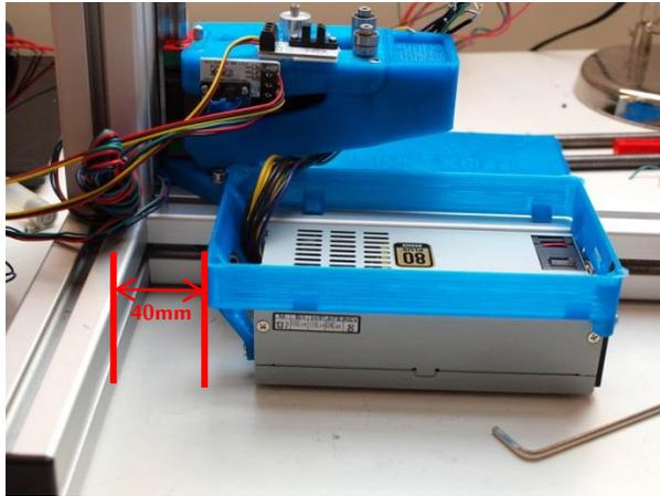
Mount the powersupply assembly onto the frame with m4x16 bolts including washers.
