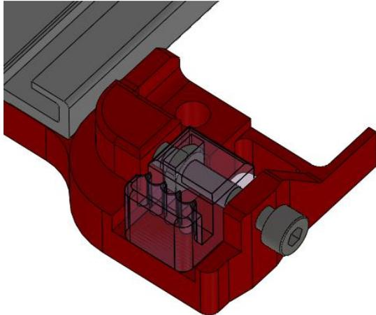
Mount the small *y-stage bracket pt4\_v4* onto the *y-stage bracket pt2\_v5\_F1\_5*. Use a m4x25 bolt and a m4 nut. This small part is needed to tension the belt later on.
