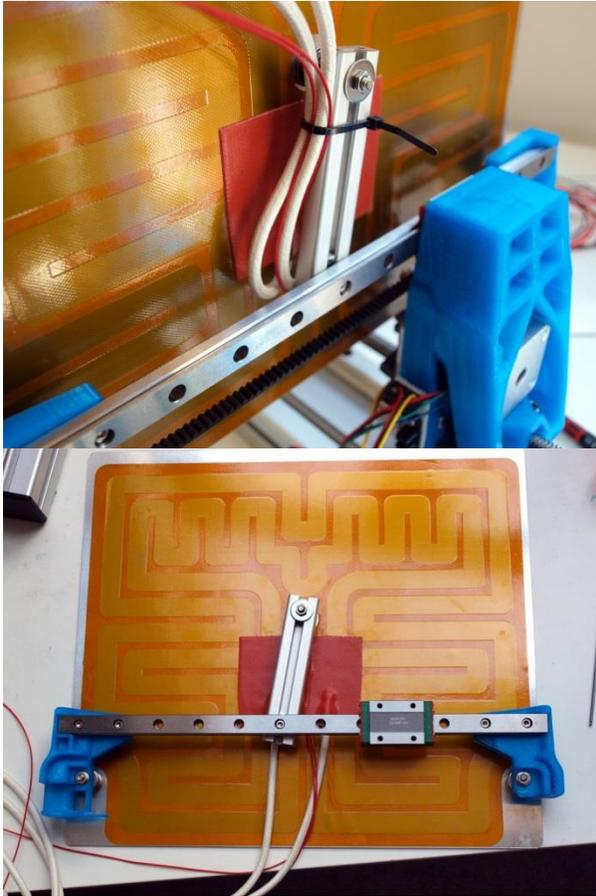
Now place the y-axis onto the table. When it doesn't directly fit, there is no need to file any parts. The three bolts can be slightly re-oriented. This can be done to exert a little sideways force on the bolt. When it still doesn't fit, you could try to adjust the position of the small aluminum beam.
