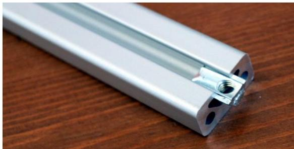
Slide in the small t-slot nut on the other side, and mount this beam onto one of the middle 2 holes of the y-axis rail with a M3x8 bolt.
