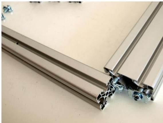
Screw the frame connectors in the bottom of beam 4 as indicated in the figure. Then slide beam 4 onto beam 1.
