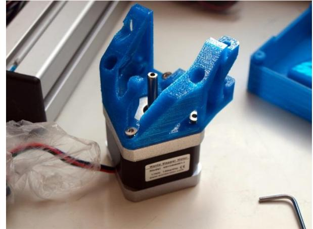
Mount the motor onto the extru\_base\_pt2 part displayed above and match the orientation of the wires.
