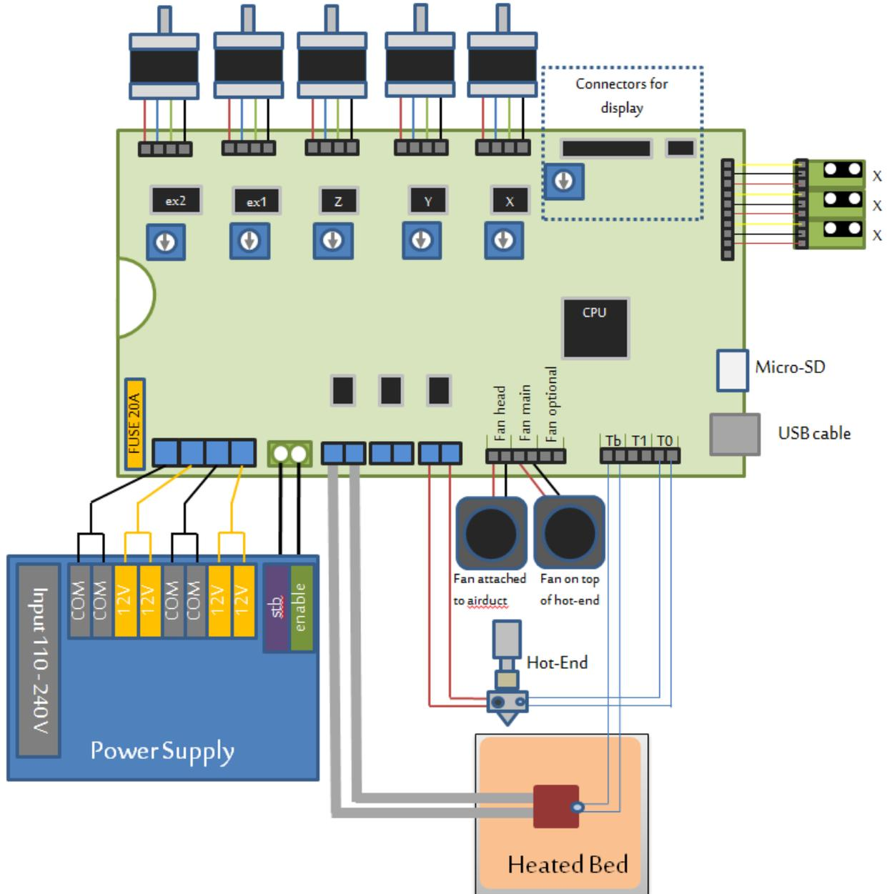
To make the printer work properly the schematics below must be matched. This chapter will guide you step by step to match the schematics above.
