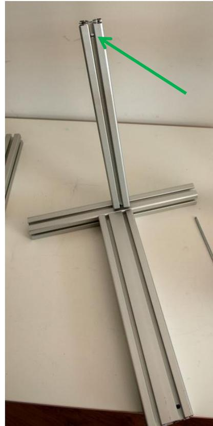
Slide one of the two beams number 2 onto beam 1. Watch the orientation of the drilled hole.
