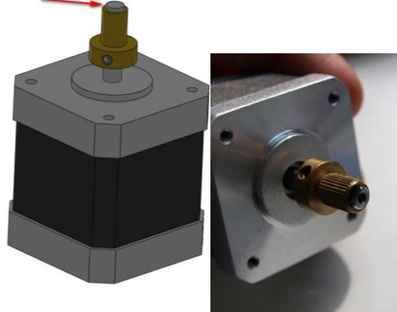
Mount the extruder wheel onto the motor with the little set-screw from the bag of the extruder wheel. The set-screw should not stick out more than 0.5mm, because it might then scrape the surrounding plastic parts..
