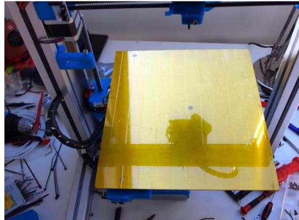
Put strokes of the supplied tape on the heated bed. Try to do this with as little bubbles and overlap of the strokes as possible. The better you do this the nicer the bottom surface of the printed parts will be.
