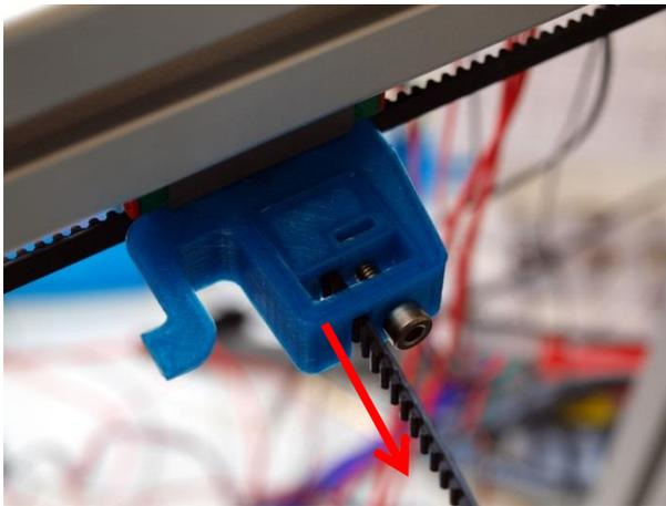
Pull on the belt as indicated above and place the small tensioning bracket in place when there is some tension on the belt. Place it just like the picture above, that there is still some room to put more tension on the bolt.
