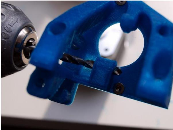
Take the extru\_base\_pt2 and drill out the hole with a 4mm drill as shown above.
