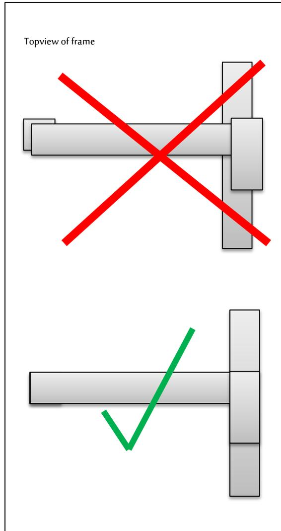
When all the beams are aligned and leveled, it is time to firmly tighten the frame connectors.
