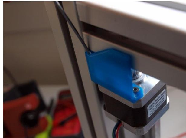
Turn the frame in its upright position and mount the motor onto the bracket. Notice the orientation of the motor.
