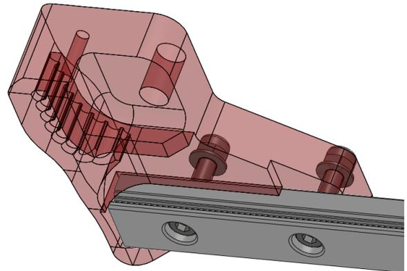
**IMPORTANT: DO NOT let the cart of the linear bearing go off the rail. There are small balls in there which might fall out when the cart rolls of the rail.**
