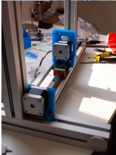
Mount the z\_axis\_carrier\_pt2\_v11\_F2\_0 onto the cart with two M5x16 bolts. Don't forget to place the m5 washers. Mount a motor onto the plastic part. **IMPORTANT: match the orientation of the wires according to the picture.**
