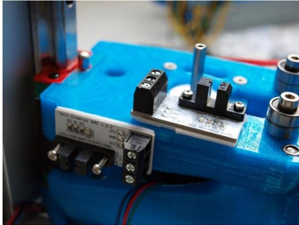
Mount the opto-sensors with the small Philips head screws. (Depending on the delivered batch it could be bronze or stainless steel screws)
