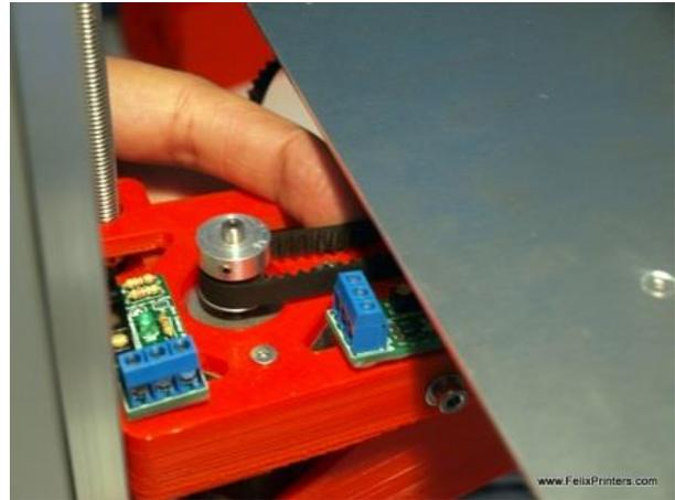
Check if you applied enough tension by pushing the belt as displayed above. It should feel firm.
