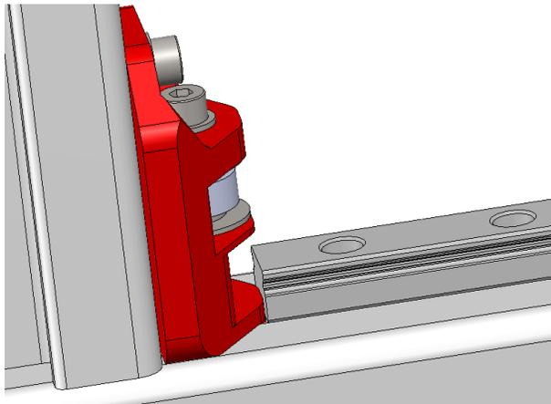
Position and fix the rail onto the frame. Let the rail touch the x-axis belt mount part.
