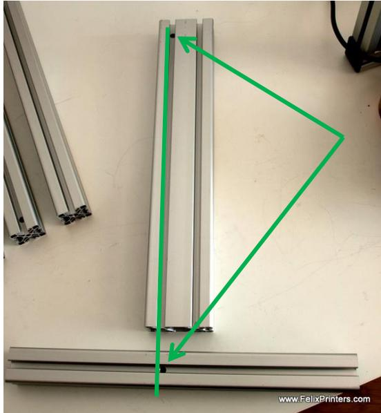
Take beam 4 and 1. They must be connected as oriented in the above picture.
