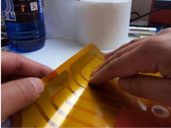
Place the sticker without bubbles on the surface. By wiping it piece by piece on the surface from the middle to the edge.
