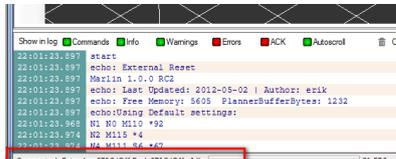
If you see **... commands waiting**, press the reset button on the side of the electronicsboard. Next to the SD card and USB connector.
