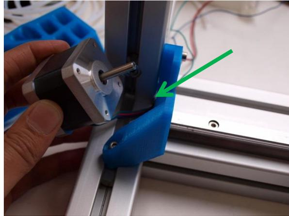
Put the motor in place and guide the wires through the hole
