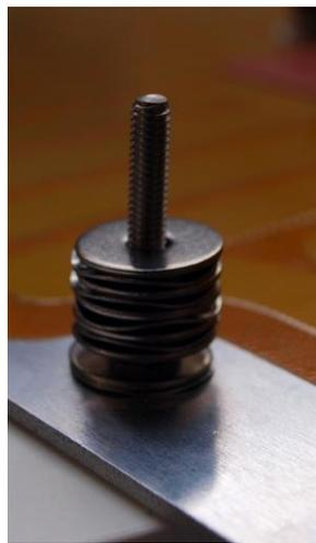
On top of the just mounted washers place per each bolt, 5 large washers and 4 curved washers.
