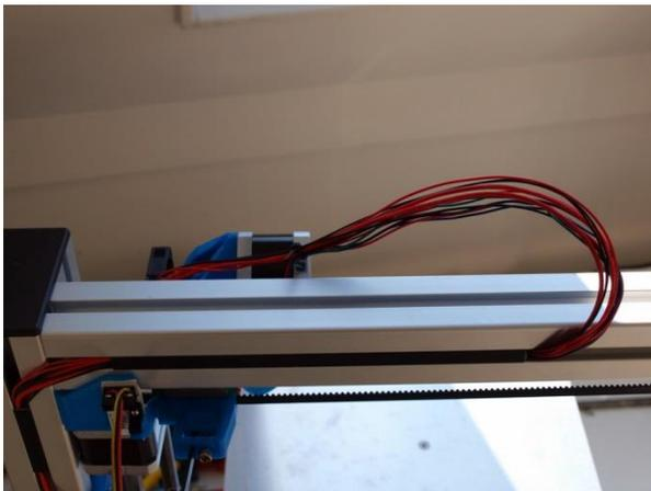
Make a nice loop for the cables which come from the extruder. It must be small/large enough that the cable doesn't get stuck around the far edge of the top beam, when the extruder is at its end position in x-direction, but there should also not be too much tension.
