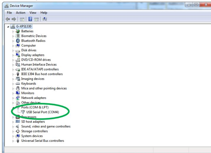
Note what COM-port is present. If there are more than one COM ports available unplug the RAMPS USB cable, and re-plug it again. Check what port number is appearing and disappearing. This port number will be used for the next step.
