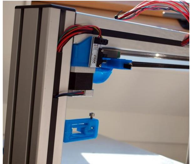
Cut off 5cm and 12cm of strip and guide the cables as indicated above.
