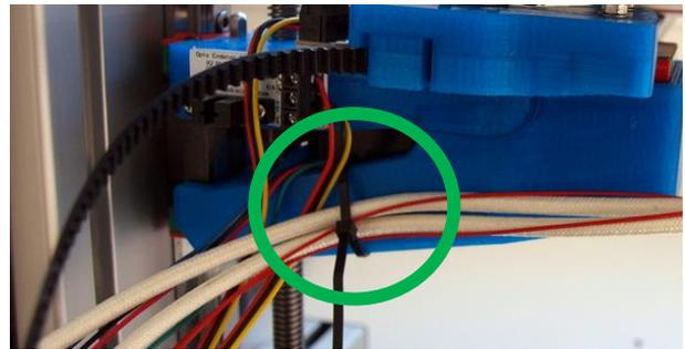
Guide the cables of the foil-heater along as shown above. Wrap a cable-tie around it to again provide tension relieve on the cable.
