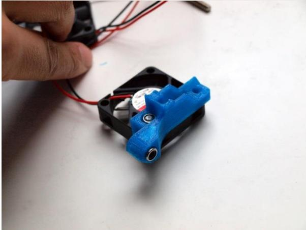
Insert the m4 self locking nuts into the hexagon holes of the extru\_base\_pt4, use an m4x20 bolt including washer as indicated above. Make sure the wires match and also the orientation of the sticker on the fan. The fan blows out air at the side of the sticker.
