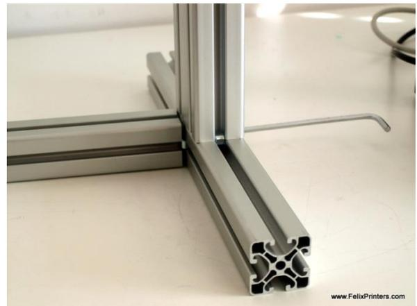
Turn the frame and fix beam 2 onto beam 1. Again not too tight.
