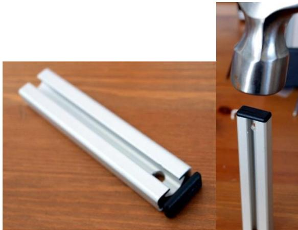
Get the small aluminum beam, first put the plastic cap on it, next to the drilled hole. This can be done with a hammer.
