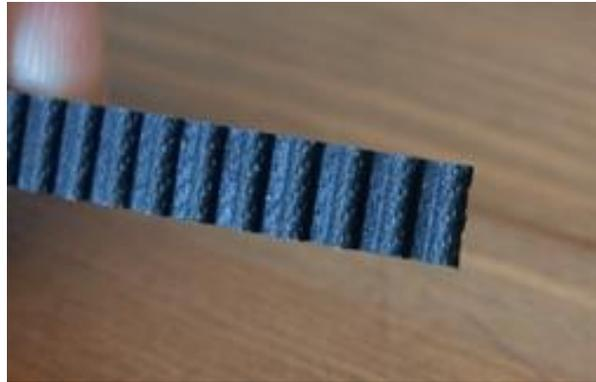
Now it is time to put the left over belt from the x-axis onto the y-axis. Take the belt and cut it off straight.
