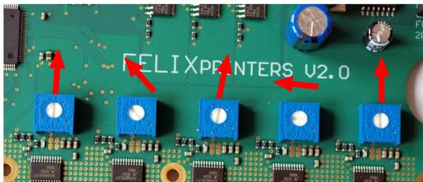
Before mounting the electronics make sure the potmeters are set ok. The pot-meters shown in the figure above regulate the power to the motors.
