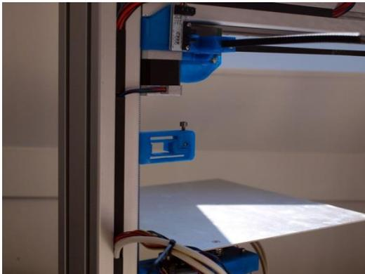
6. Mount the frame handle. Use the supplied M8 (or M6 frame nuts depends on the handle type delivered) and bolts to mount it. Place the frame holder as close to the vertical frame beam as possible.
