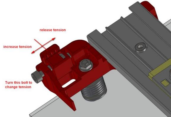
Next step is to tension the belt by turning the tensioning bolt. See picture above. The belt should be tensioned when the distance between the parts is approx. 1 to 2 mm.
