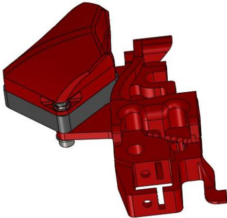
Mount the fan and airduct with m4x20 bolts onto the extruder base. Use m4 selflocking nuts and also use washers. The bolts don't have to go all the way through the self locking part of the nut.
