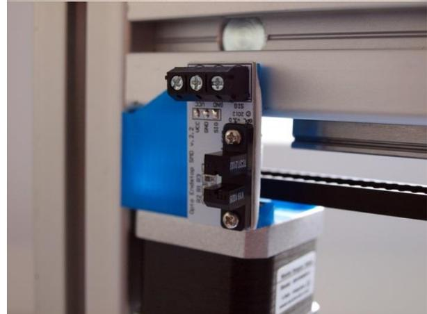
Put some double sided tape on the opto-sensor and mount it onto the bracket with the small philipshead screws.
