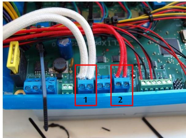
Connect the heater wires of the bed and hot-end
