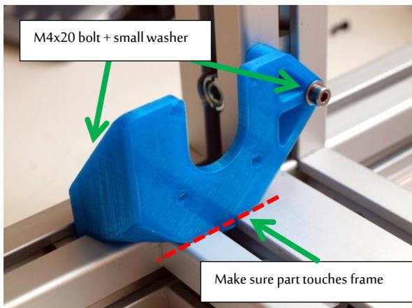
First mount the linear guide loosely onto the frame with M4x20 bolts. Then mount the *z-axis-motor-bracket\_v10\_F2* onto the frame, indicated above with m4x20 bolts and important use small washers.
