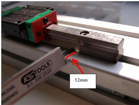
Start to align the z-axis guide. Push the bottom side against the printed part. Measure the distance of the edge as indicated above. The distance should be 12mm.
