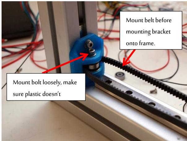
**IMPORTANT MOUNT THE BELT BEFORE MOUNTING THE BRACKET SHOWN ABOVE:** Guide the belt over the bearing as shown above before mounting the sub-assembly to the frame. The top-bolt in the picture is an m4x16 bolt, also use a washer.
