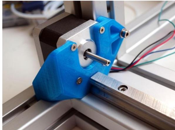
Mount a motor with the m3x8 CSK (countersunk head) bolts.
