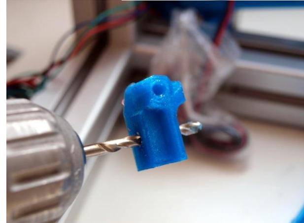
Get the extu\_arm part and clean out the hole with a 4mm drill as shown above slowly.
