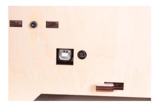
The reset switch is on the back of your Creator, just to the right of the USB port. You'll probably also need something to press the button with -- most fingers won't fit. Hit the upload button, press the reset button, and wait
