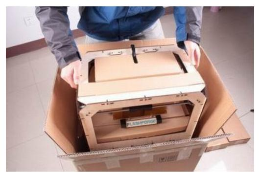
You should be able to see the build platform: it's an aluminum plate covered in Kapton tape and attached to the rods by two black plastic arms. This is where your prints will form. Note: Do not remove Kapton tape, it help object stick to plate firmly.
