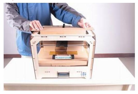
You'll need to raise the platform to finish unpacking. You can either turn the threaded screw, or grasp the build platform firmly on both sides and move it up with gentle pressure.
