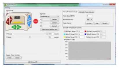
On the left side of the control panel window, you can use the axis buttons superimposed on the image of your Creator to move each axis. The labels are arranged to match the direction of movement that you'll see on the bot, and the plus or minus matches the direction you'll see in the GCode. We highly recommend the "Continuous Jog" setting here, but you can also move the axes by predetermined increments.
