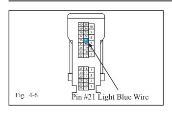
(g) Locate the LIGHT BLUE wire (pin #21) on the 3C 40-pin connector. (Fig. 4-6)
