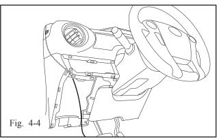
(e) Route the harness from the bottom of the a-pillar through the opening on the back of the dash, and out through the opening on the lower dash panel.
