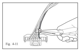
(l) Attach the RED T-tap connector to RED wire (pin #8) with needle-nose pliers. (Fig 4-11)
