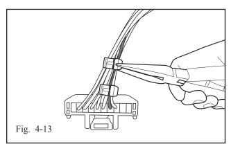
(n) Attach the RED T-tap connector to WHITE w/BLACK TRACE wire (pin #7) with needle-nose pliers. (Fig 4-13)
