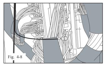
(i) Plug the BLACK wire spade with BLUE marking on spade end of the EC mirror harness T-tap connector on LIGHT BLUE (pin #21) wire. (Fig. 4-8)
