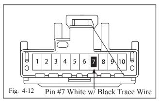
(m) Locate the WHITE w/ BLACK TRACE wire (pin #7) on the G7 10-pin connector. (Fig. 4-12)
