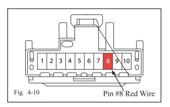
(k) Locate the RED wire (pin #8) on the G7 10-pin connector. (Fig. 4-10)
