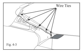
(d) Route the harness down the a-pillar, and secure to the OEM harness with (5) five wire ties. (Fig. 4-3)
