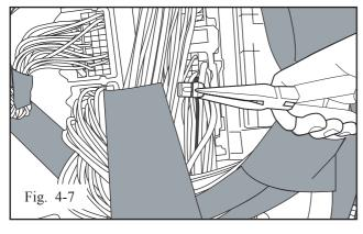
(h) Attach a RED T-tap connector to LIGHT BLUE wire (pin #21) with needle-nose pliers. (Fig 4-7)
