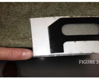
Remove Liner off bottom of the part leaving white Template on part intact as shown.
