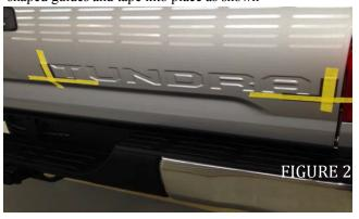
Remove alignment tool leaving magnetic guides taped in place.
