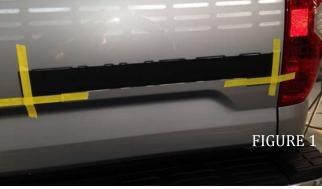
Place Magnetic Alignment tool on Tailgate, install L shaped guides and tape into place as shown
