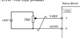
Programmable controller and so on are used for connection with the instruction controller's speed instruction output terminal in case of position control by instruction controller.
