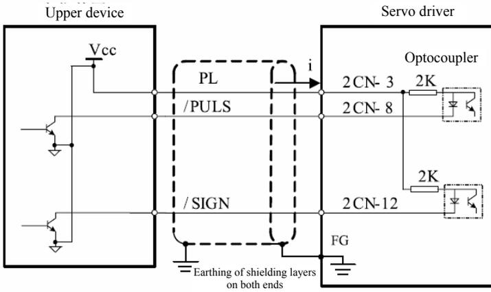
b) When the upper device adopts open collector output and provides 5VDC, 12VDC and 24VDC signal power supply, the connecting type is 2.
