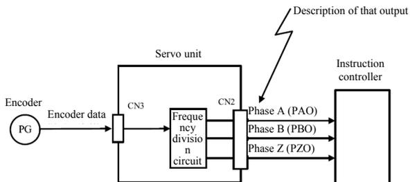
Note: The width of original point pulse is fixed and irrelevant to frequency division ratio.
