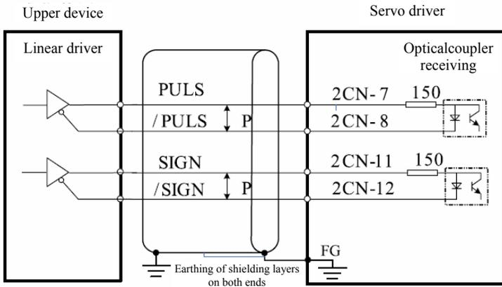
b) Driver receives through high speed pulse channel
