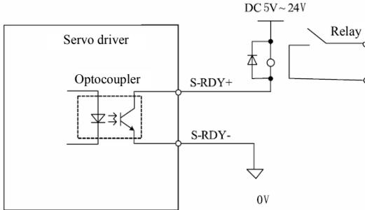
(note) The maximal allowable voltage and current capacity of the output circuit of optocoupler is as follows:
