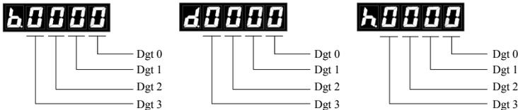
b: means binary system display setting, digit value setting range: 0 ~ 1;
