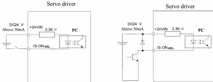
Take the above figure as an example. When the opticalcoupler is conductive, S-ON signal is L level; when the opticalcoupler is not conductive, S-ON signal is H level. Parameter PA508 decides the active level of S-ON. When PA508.0=0, S-ON signal is L level active; when PA508.0=1, S-ON signal is H level active.
