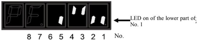
The input optocoupler is not conductive, PA508.0 = 1, and S-ON signal is inactive (servo ON at H level).
