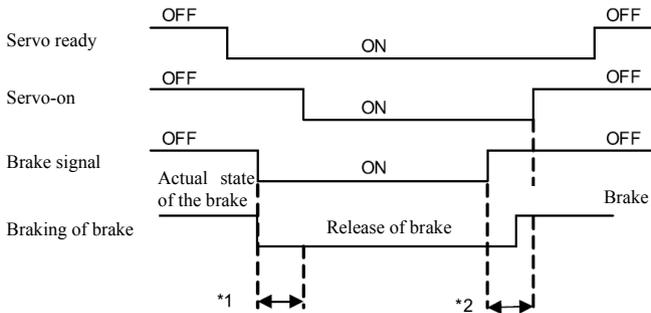
\*1. The time from brake signal active to brake release is different for different types of brake.
