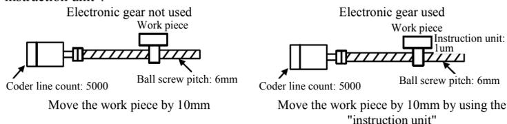
As one turn is 6mm, to move 10mm, you need to rotate by  $10 \div 6 = 1.66667$  turns; As rotating by 1 turn needs to use  $5000 \times 4$  pulses, so the instruction needs to input  $5000 \times 4 \times 10 \div 6 = 33333$  pulses. This computation must be conducted on instruction controller.
