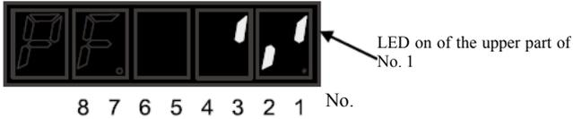
PA511.0=1, ALM signal L is active, and the opticalcoupler is conductive (ALM signal is L level)
