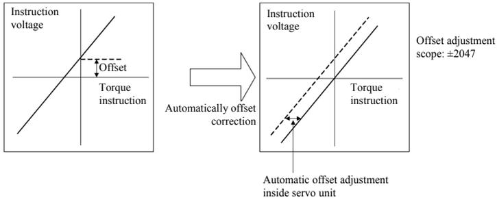
Once automatic adjustment of instruction offset is implemented, that offset will be stored inside servo driver.
