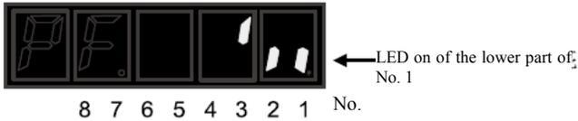
PA511.0=0, ALM signal H is active, and the opticalcoupler is not conductive (ALM signal is H level)
