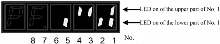
The input optocoupler is conductive, PA508.0 = 1, and S-ON signal H is inactive (servo ON at H level).
