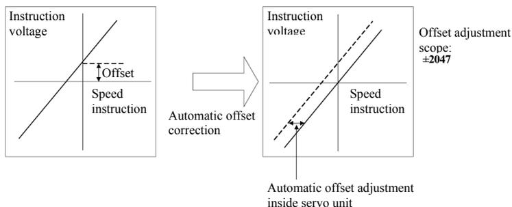
Once instruction offset is automatically adjusted, the offset will be stored inside servo driver. The offset can be confirmed through manual adjustment (AF007) of speed instruction offset. Please refer to “8.5.3(2) Manual adjustment of speed instruction offset”.
