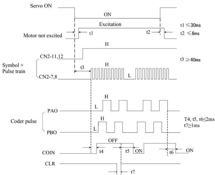
(Note) 1. The duration from servo ON signal is set to ON to instruction pulse is input should be controlled to above 40ms. If instruction pulse is input within 40ms since servo ON signal is set to ON, servo driver sometimes can't receive the instruction pulse.
