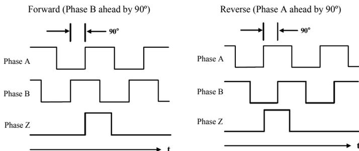
Please make servo driver rotate by two turns before using servo driver's phase Z pulse output for mechanical original point reset action.
