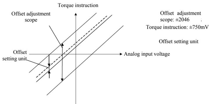
Please adjust the torque instruction offset manually according to the following steps.
