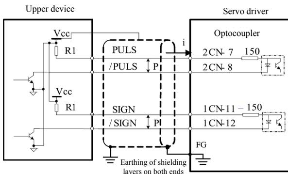
Please select the value that limits resistor R1 to ensure that input current  $i$  is within the following scope:
