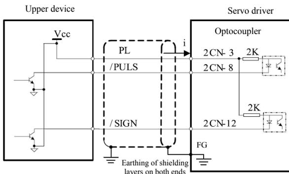
When collector power is 12V or 5V, connection can be done according to the following chart:
