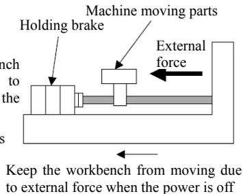
1. The brake of the servo motor with a brake is special excitation-free action type holding brake; it can not be used for braking, and can only be used to maintain the halt state of the servo motor. The brake torque is about 80% of the rated torque of servo motor.
