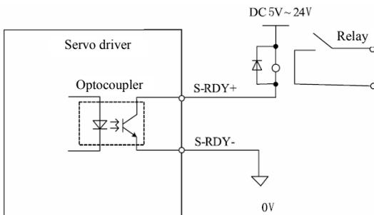
(note) The maximal allowable voltage and current capacity of the output circuit of opticalcoupler is as follows:
