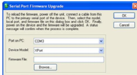
2. Power off the device. Connect a serial cable from the PC running the DeviceInstaller to the primary serial port on the device.
