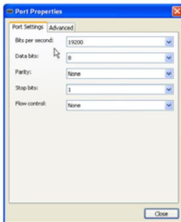
3. The Port Settings window displays general serial port settings. Select the **Advanced** tab to configure advanced serial port settings.
