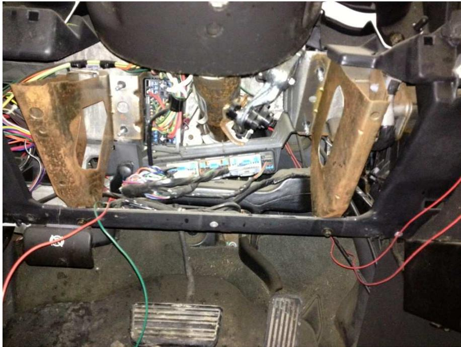
4. Mount the main control box securely under the dash so the wires have enough slack to properly reach the driver side fuse block. It can be zip-tied in place, or secured with double sided tape. **NOTE: BE SURE TO DOUBLE CHECK THAT MOUNTING OF MAIN CONTROL BOX AND ASSOCIATED WIRING DOES NOT INTERFERE WITH ACCELERATOR/BRAKE PEDAL MOVEMENT OR STEERING COLUMN MOVEMENT. ALSO USE EXTREME CAUTION AROUND ANY YELLOW/ORANGE COLORED CONNECTORS, AS THESE ARE AIRBAG SYSTEM RELATED CONNECTORS AND WIRING.**
