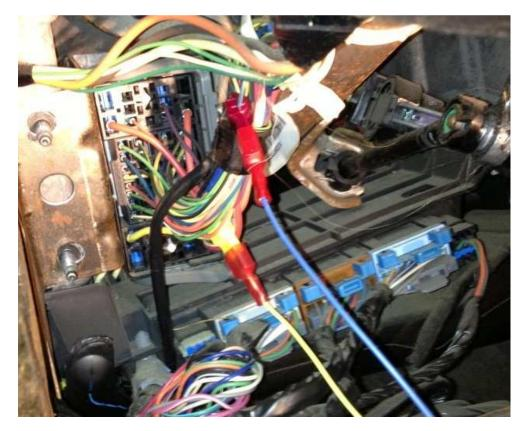
12. Locate the DARK-GREEN/WHITE-STRIPE wire on the brake pedal switch connector. You may have to unplug the connector to get a better view of it.
