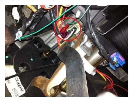
15. Locate the driver side footwell junction block. Remove the cover, and locate the large brown square connector as shown.
