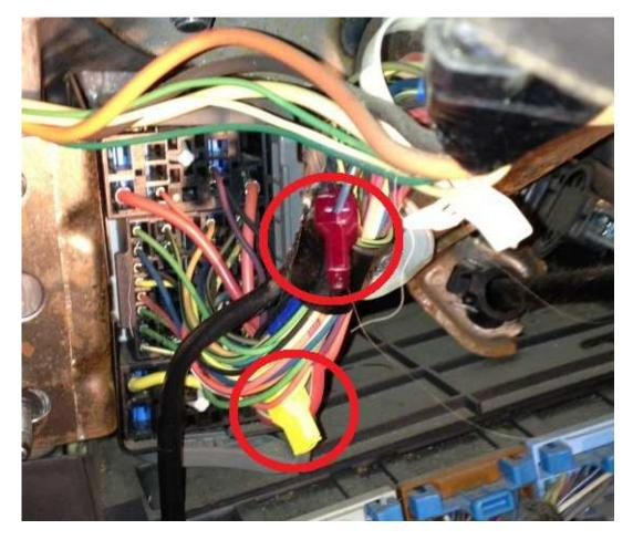
11. Connect the YELLOW wire coming from the high-idle module to the YELLOW wire that you just crimped the wire-tap onto, and connect the DARK BLUE wire coming from the high-idle module to the DARK BLUE wire that you just crimped the wire-tap onto, as shown.
