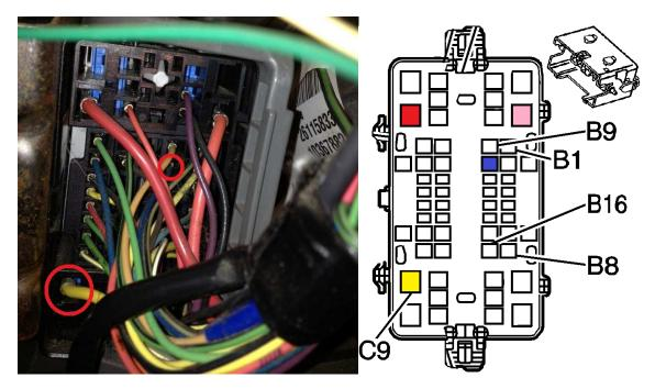
9. Crimp the yellow wire-tap onto the thick yellow wire as shown.
