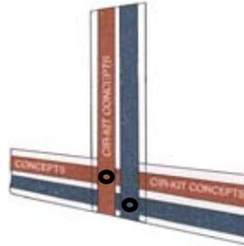
**The Ceiling Run:** Begin at the base run of the desired room and run up the wall and across the ceiling. Attach this new run to the baserun with 2 eyelets. An adapter will be used to attach the ceiling light to the tapewire at a later time. Lightly spackle and paint or cover with a ceiling paper.
