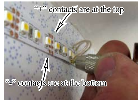
Punch a hole in a "+" contact and a "-" contact. Remember the first photo? The blue lead ("- in this house) was toward the back. So the back wire is going to the "-" side of the ExtraBrite® Striplight, which is at the bottom here. Insert the wire and secure with an eyelet (don't hit the emitter with the end of the tool).
