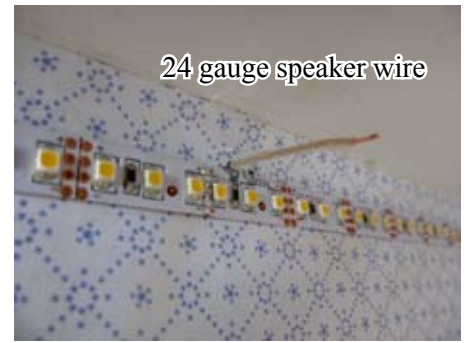
Strip both ends of a short piece of wire. Poke an end into the hole.
