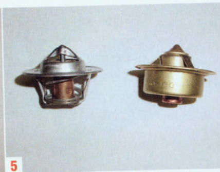
5 A conventional thermostat on the left, and a balanced-flow type on the right; the balanced-flow type is more accurately calibrated.
