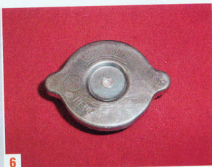
6 The radiator cap, which maintains system pressure, vents overflow, and admits air on cooldown. Most auto parts stores can verify its seal and pressure calibration.
