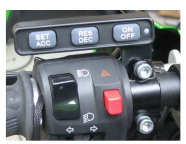
The **Control Switch (5)** is mounted to the left hand (clutch) master cylinder handlebar clamp. The bracket mounts between the upper faces of the clamp and the master cylinder. The clamp must have about  $2.0 \text{mm} (0.080^{\circ})$  filed from the top face to allow for the thickness of the switch bracket.
