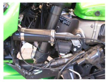
The **Electric Throttle Servo (2)** mounts under the left side fairing panel. This photo is taken with the left side fairing panel removed. A cable runs from the servo to the Cable Interface Unit.
