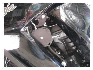
This photo shows the throttle servo and CIU with the fairing panels removed.
