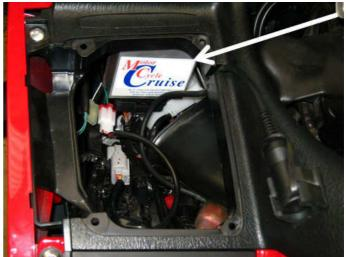
The **Electric Throttle Servo (2)** is mounted in the right side of the fairing, below the right audio speaker, above the radiator. A special bracket is supplied to mount the servo. A **servo cable (3)** connects the servo the vehicle's throttle body.
