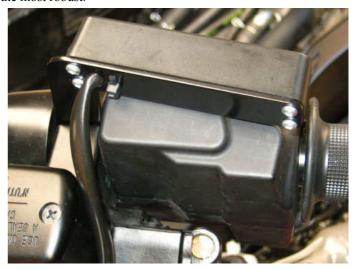
An **OPTIONAL** mounting arrangement is available for the **Control Switch (6).** This arrangement places the control switch in a similar position, but it is screwed to the removable top cap of the bike's left side switch block. The bracket is cut to 'fit' the top of the bike's switch block. This requires that 2 holes are drilled in the cap. This is still fairly easy to install, but requires partial disassembly of the bikes left hand switch block to fit it.
