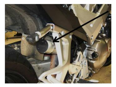
The CIU (3) is located on the left side of the bike, above the rear corner of the radiator. It is hidden inside the fairing. A new cable (4) connects it to the throttle bodies.
