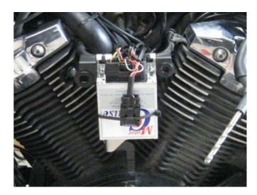
The **Actuator** (2) is mounted on the front left side of the engine, mounted on the frame down tube using hose clamps around the frame tube (lower left corner of the photo). Satin Black powder coated aluminium covers are supplied to prevent dirt and water ingress into the actuator and to improve the appearance of the actuator. A **vacuum hose assembly (3)** is provided to connect the actuator to the engine.
