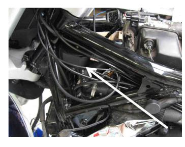
The Control Switch (6) is mounted on the left side mirror stalk.
