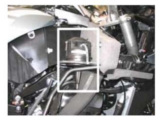
The **Cable Interface Unit (5)** is located on the left side of the motor, near the front left corner of the engine. It has a new **cable (6)** running from it to the fuel injection throttles. The computer (1) is also shown in the photo below left. The photo below right shows the CIU with the fairing fitted to the bike.
