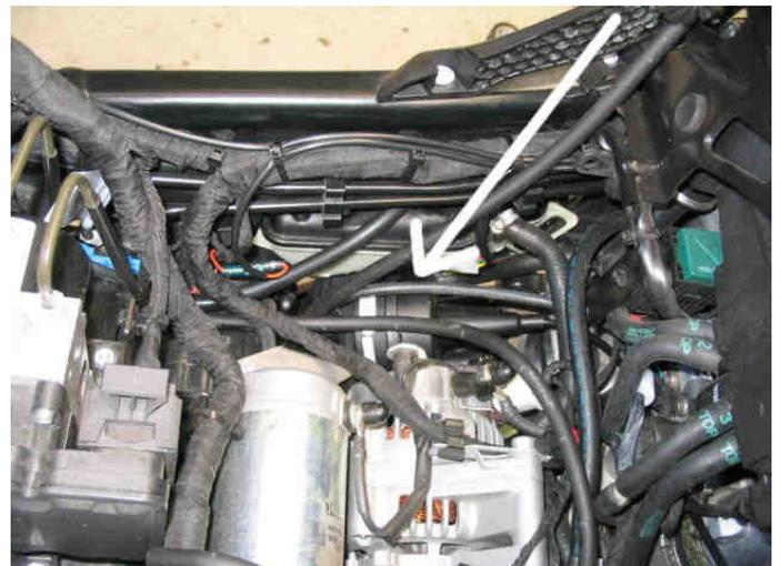
The **CIU (4)** is located on the right side of the bike above the radiator. It is fully covered by the fairing panel. A new **cable (5)** connects it to the throttles. The photo at right shows the CIU viewed from the front of the bike with the fairing installed. These photos are of a K1200S, but the K1300S installation is almost identical.
