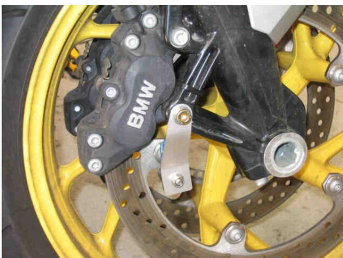
The **Speed Sensor (6)** is mounted below the right hand front brake caliper. The original caliper mounting bolt is removed and a new bolt and spacer washers fitted to allow the speed sensor to be mounted. Nickel-plated magnets are placed in the heads of the bolts that mount the brake disc. **NOTE: - See the note at the end of this document regarding different magnet sizes in BMW brake disc mounting bolts.**
