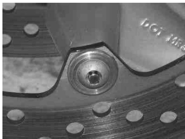
Note that these bolts are used in earlier designs that bolt a disc carrier to the wheel and the discs then are allowed to 'float' on the carrier and also later models as shown here with the disc bolted to the wheel without a carrier, but there are spring washers on the bolt to allow the disc to 'float'.
