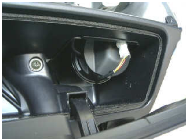
A close up of the actuator (2) in the fairing pocket (photo at left).
