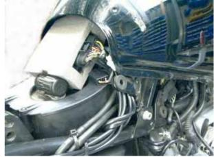
The **Actuator** (3) is bolted to the right side of the gearbox, using the right footrest mounting bolts. Silver Pearl (shown) or Satin Black (optional) powder coated aluminium covers are supplied to prevent dirt and water ingress into the actuator and to improve the appearance of the actuator. A **vacuum hose assembly** (4) is provided to connect the actuator to the engine.
