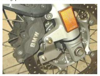
The **Speed sensor** (7) is mounted below the right hand front brake caliper. The original caliper mounting bolt is removed and a new bolt and spacer fitted to allows the speed sensor to the mounted. Nickel-plated magnets are placed in the heads of the bolts that mount the brake disc.
