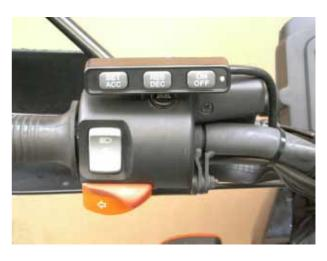
disengage the cruise if the clutch is operated. The bike's clutch switch is also connected to the cruise control to disengage the cruise control. These connections require the wires to be spliced to the bike's wiring loom because we have been unable to source the connectors used on the bike. The cruise control is grounded on the battery negative terminal.
