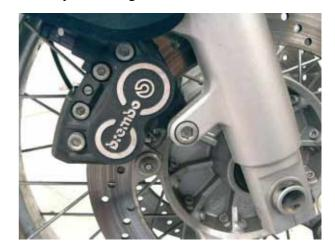
Later models were fitted with the Evolution brake package. This included these calipers, labeled with the BMW logo.
