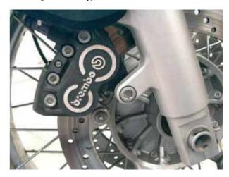
Later models were fitted with the Evolution brake package. This included these calipers, labeled with the BMW logo.
