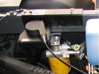
The **Throttle Lever (4)** is located on the right side of the transmission and controls the vehicle's hydrostatic transmission. The new lever and other hardware bolt directly to the vehicles throttle mechanism.
