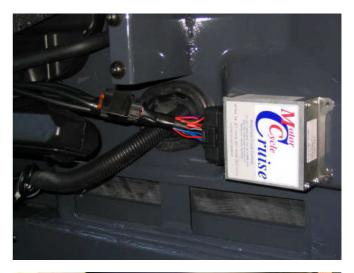
The Electric Actuator or throttle servo (2) is mounted inside the engine bay on the left side, using two bolts that mount the filter. An Actuator cable (3) connects the actuator to the vehicle's throttle mechanism (see next page).
