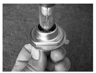
Cut off the two smaller mounting tabs with tin snips, large scissors or other suitable tool.
